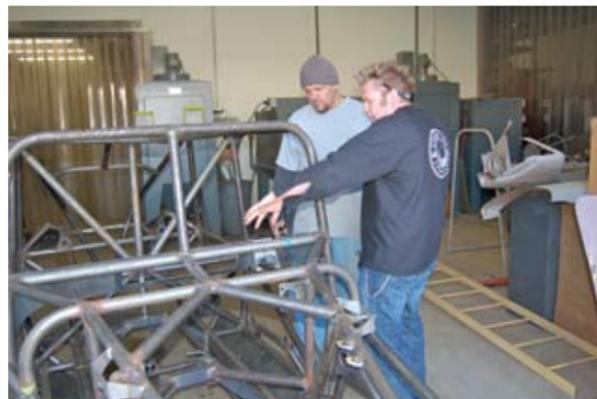
Josh and I spent a good hour or so talking about the plan for the coating on the chassis. Determining what sections would receive custom masking, and what sections would just get a color coat. This attention to detail is what gives Streetwerkz their reputation as a high end powder coater.
