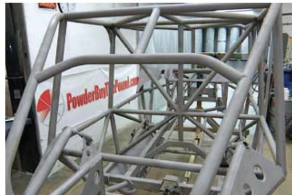
A primer coat was then applied to the chassis to act as a base for the first color coat. This evens out the color of the base and ensures that any difference in base material color does not transfer into the top coat.
