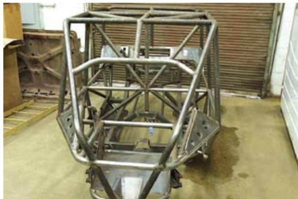
With the design laid out, and the masking locations planned, the first step was to degrease the entire chassis. Just like a high end paint job, the prep is one of the most important parts of this process. My good friend Kevin Tetz, a pretty hot shot painter in his own right, often compares paint prep to eating liver, in order to get dessert.
