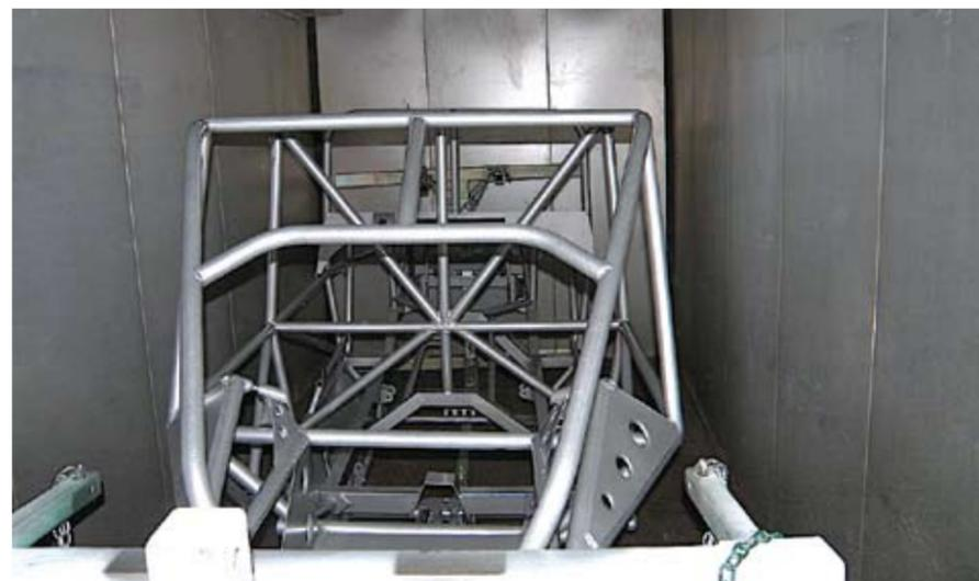
The second coat of "silver" was applied then the chassis is put into the oven at 400 degrees for 10-15 minutes, and the powder liquefies. The melting powder creates a "shell" around the metal it has been sprayed onto, making it stronger than a typical painted finish.
