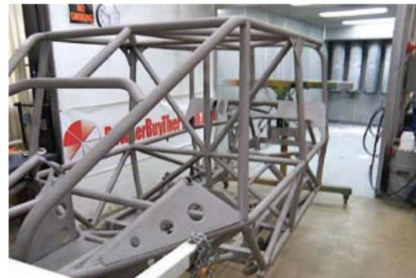
The powder was applied to the chassis in a large spray booth; sprayed from the gun with a positive static charge on the powder. The powder is attracted to the chassis because of the attraction between the positively charged powder and the negatively grounded chassis. A silver base was the first layer of colored powder, and the start of the candy blue finish.
