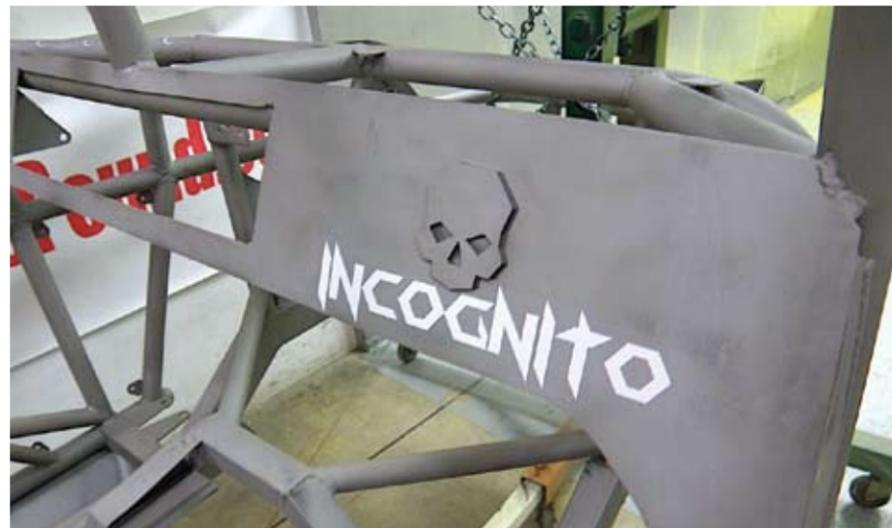
Masking was used to create a custom design on this buggy, different than any other buggy you might find on the trail. By using a temperature safe masking coating that is cut by a local sign shop, StreetWerkz can take any design you can think of, such as your shop name, custom designs or images, and apply it to the buggy.
