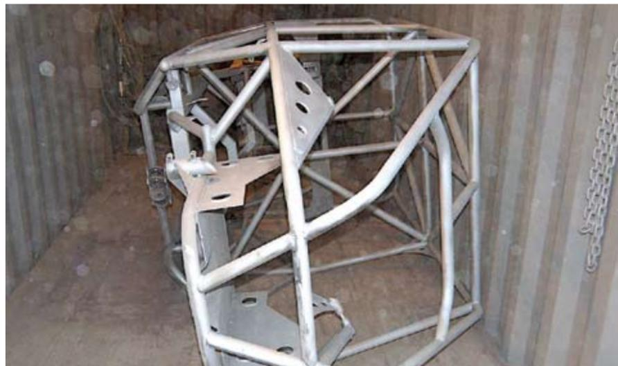
With the chassis secured to the rack, it was ready for the powder to be applied. The location of the grounding wires is key; ensuring the electrically charged powder becomes attached by providing the current flow of the grounding circuit to promote the powder's adhesion to the chassis.
