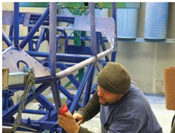
Block sanding the chassis “leveled” out the final coats of clear. This is essential on a project that has multiple layers, and has the “ghosted” images buried under multiple layers of powder.
