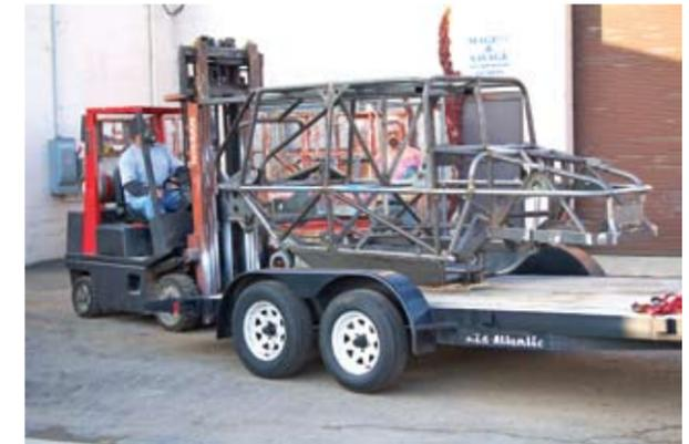
I rolled into Columbus with my chassis stripped down, and completely finish welded from front to back. It took 24 hours of fitting, grinding, and welding to prep this complete four seat chassis.
