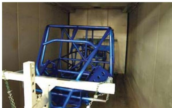
After each coat of candy blue, the chassis was baked in the oven until the chassis reached 400 degrees. Each coat of the semi transparent blue made the final candy coat darker, and when the desired color tint was reached, the chassis was ready for clear coat.
