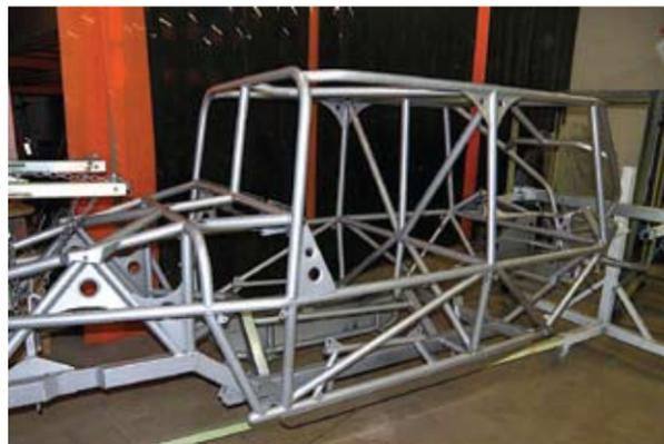
Once out of the oven, the chassis is checked to ensure that the base color has sealed all the raw metal. The base silver is allowed to cool, and the masking is removed to create the “ghosted” image. This is where all the time spent laying out over 250 linear feet of custom graphics really starts to pay off.
